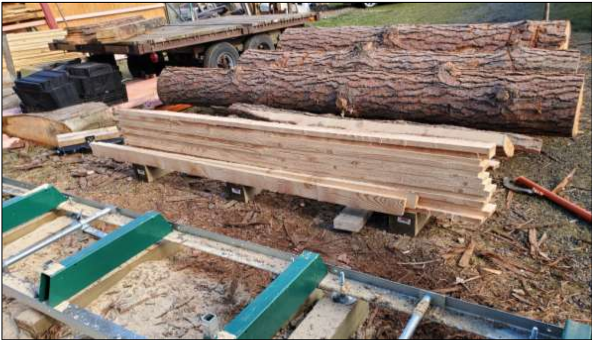
Figure 14: The saw logs at Daniel's mill, and the stack of 1x4s that he milled from the first two!.
